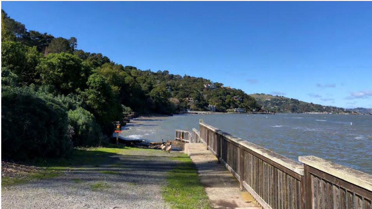
Figure 41: Photograph looking down the boat ramp that leads to the intertidal area where the proposed beach would be built. The photograph was taken at a tidal level of +5 ft which is below the MHHT level of 5.84 ft, our design water level. Note that none of the beach area at Paradise Cove park is accessible during high tide conditions. The beach designs will fill this area at the end of the ramp with a gravel beach.
