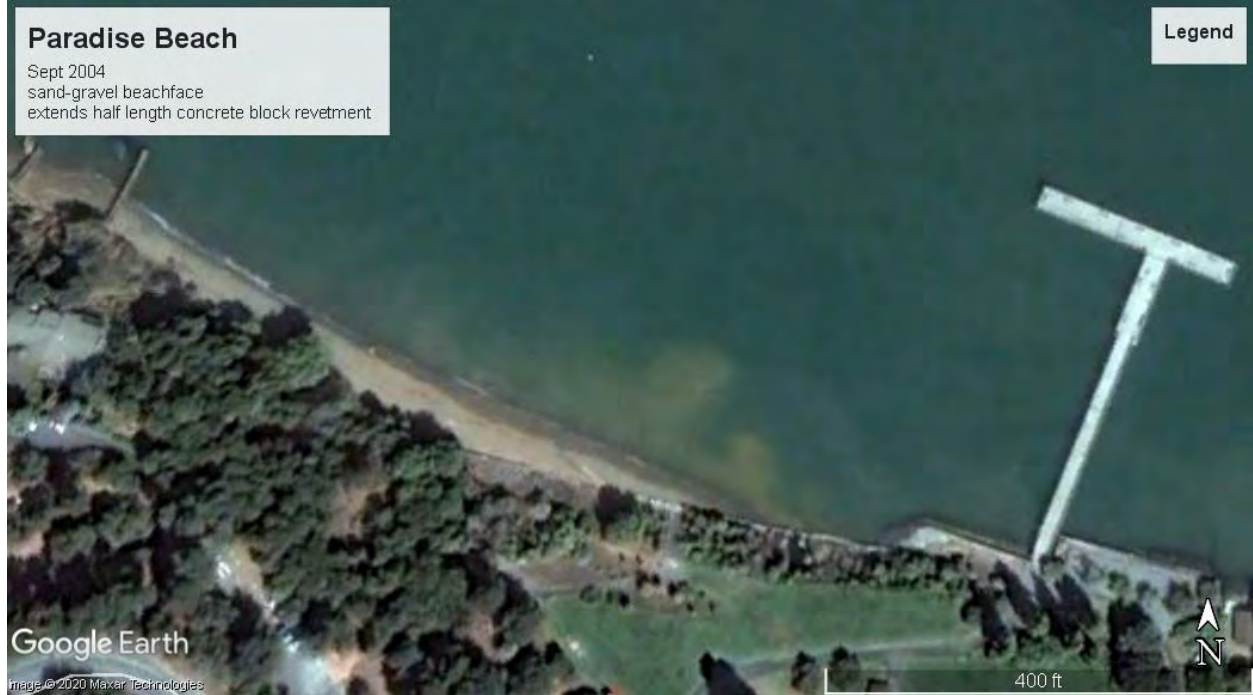
Figure 35: The gap between the sand-gravel beach and the old concrete boat ramp in Sept 2004 and May 2009 was small (less than 150 ft) at mid-tide. In 2019, it was close to 280 ft wide because of beach erosion.
