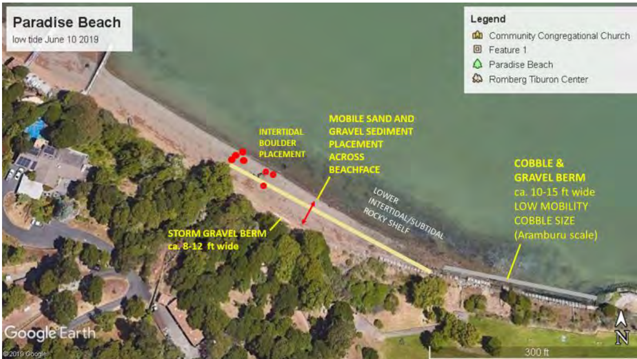
Figure 31: Approximate plan view layout of Alternative 2 conceptual design over Google Earth low tide image of Paradise Beach (June 2019), with scale.
