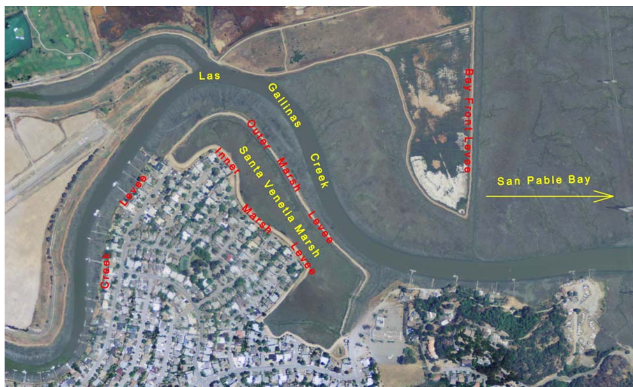
Figure 6-1. Inner/Outer Marsh Levees, and Bay front Levee Blocking Bay Waves
