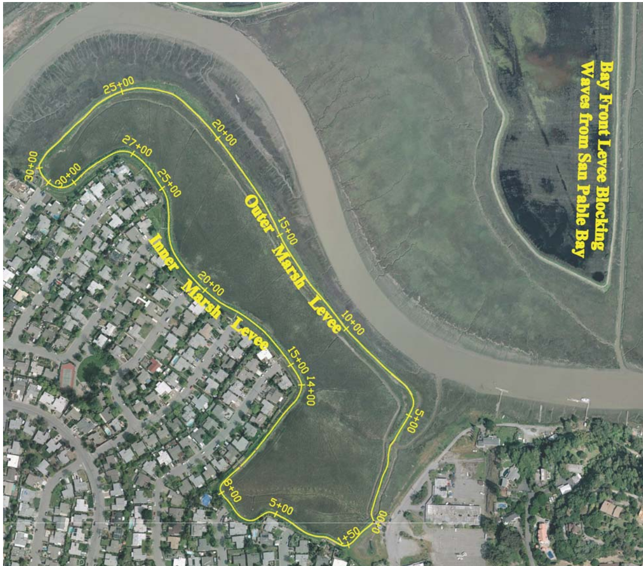
Figure 6-4. Stationing of Inner and Outer Marsh Levees
