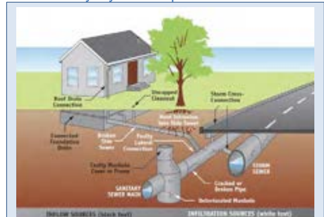
Figure 4. Inflow and Infiltration Sources to the Sanitary System Pipeline
