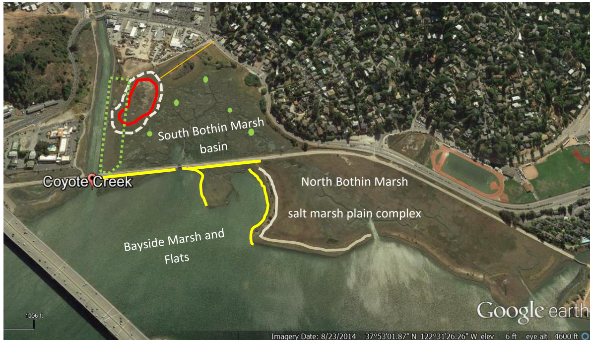
Figure 5: Conceptual Layout of Bothin Marsh Preliminary Eco-geomorphic Units and Major Project Components
