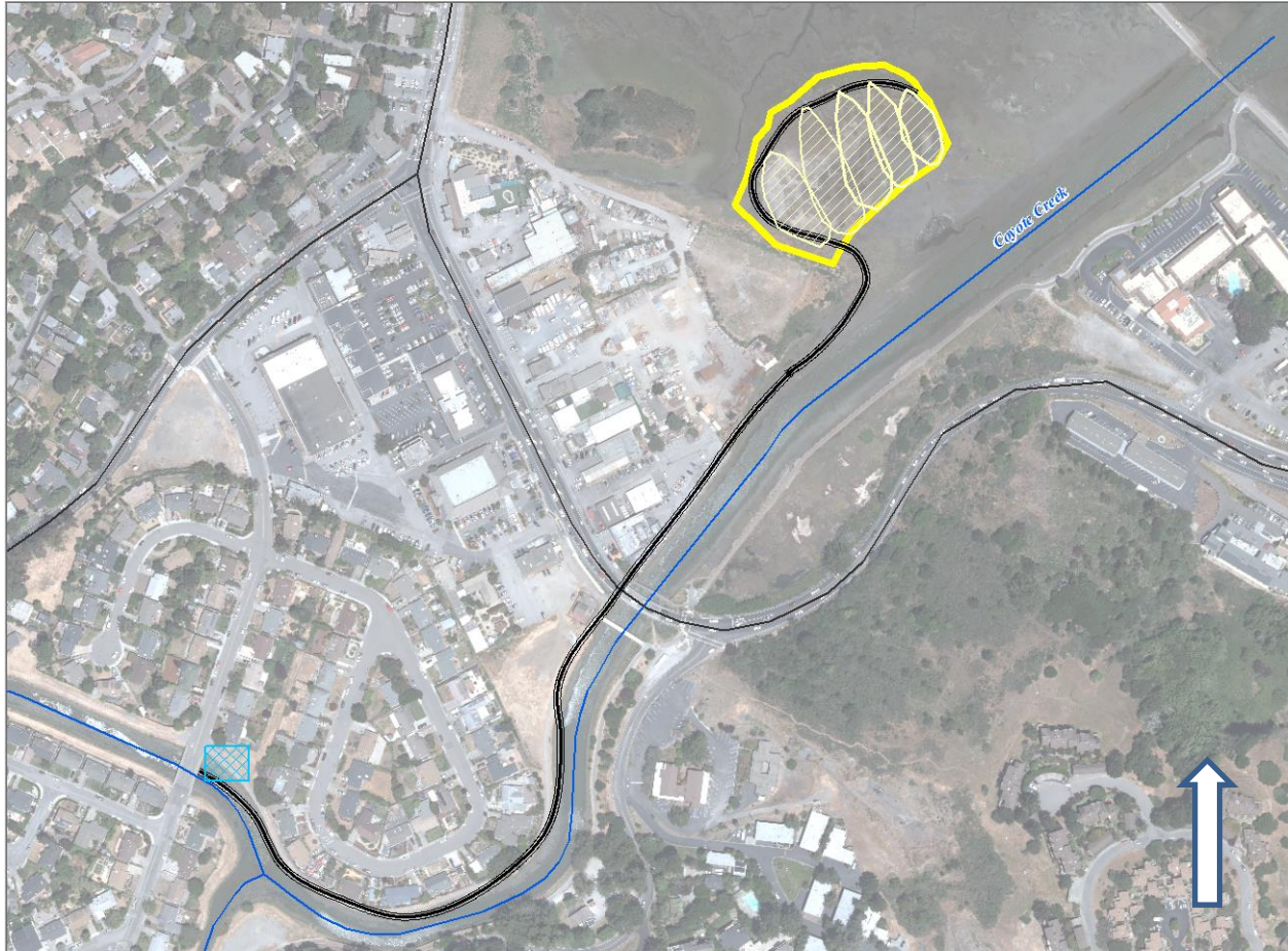
Figure 8: Schematic Location of Hydraulic Dredge Pipeline(blue hatched rectangle at upstream is the likely furthest location up the channel of the hydraulic dredging operation). The reach from Flamingo Road Bridge upstream to the concrete channel is assumed to be dredged mechanically using an excavator on the adjacent levee.
