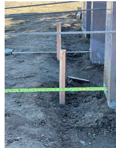
Figure 5. Deflection measurement at the rear and front of wall left and right photographs respectively. Dynamometer shown in center photograph at 17,660 pounds.
