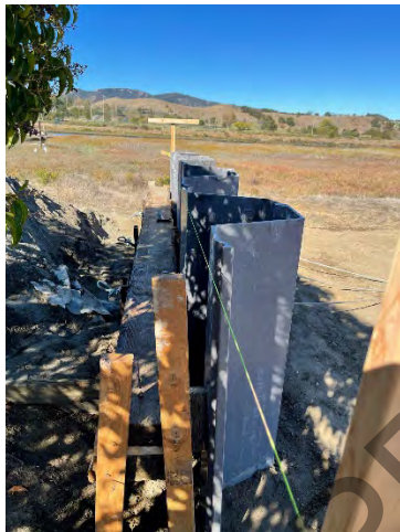
Figure 5. Deflection measurement at the rear and front of wall left and right photographs respectively. Dynamometer shown in center photograph at 17,660 pounds.
