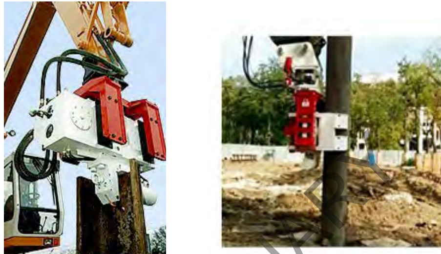
Figure 25 Sheet pile installation tools including a top grip on the left and side grip on the right.
