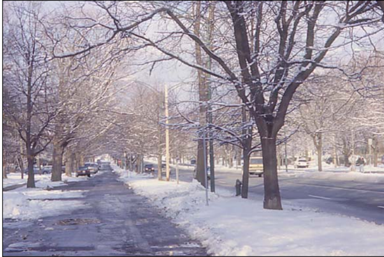
Figure 9.25 Snow is stored in the median of this multi-way boulevard in Albany, NY. Source: Community, Design + Architecture.
