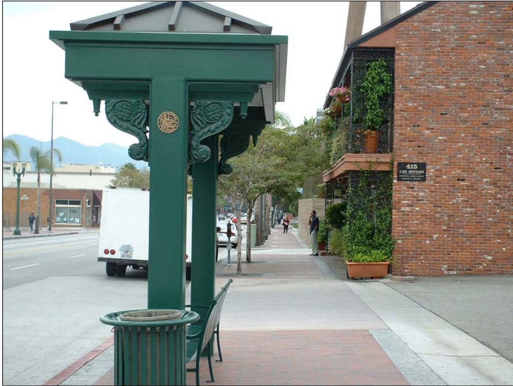
Figure 8.6 Utility poles and other fixtures should not interfere with the pedestrian thoroughway. This example shows a bus shelter and other street furniture properly located in the furnishings zone. Source: Kimley-Horn and Associates Inc.
