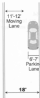
FIGURE 2-15 Street and lane widths.
