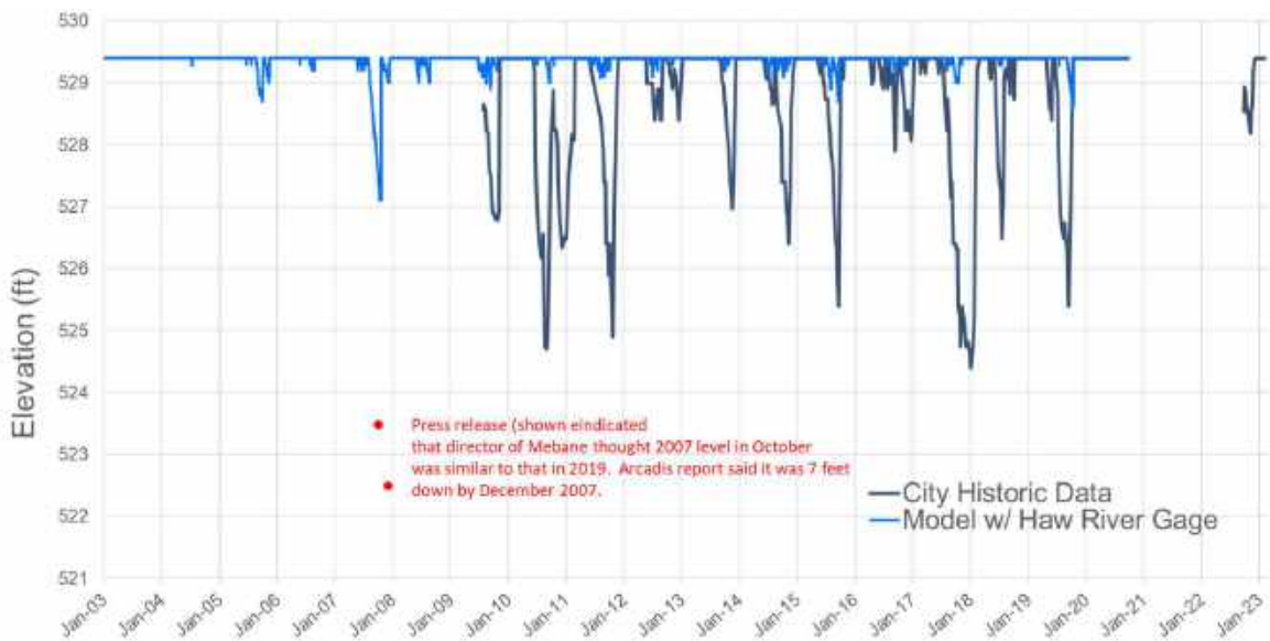
Figure 4-7: Verification Test Using Inflows Based on Haw River Gage @ Haw River, NC
