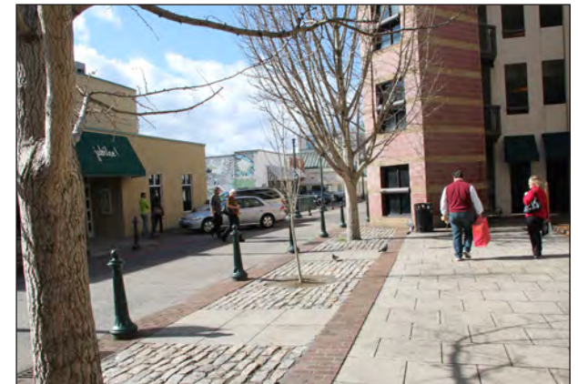
Shared Pedestrian/Vehicular Alley in Asheville. This alley is all at the same elevation, with cars separated from pedestrians with bollards.
