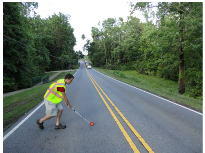
A consultant measures roadway dimensions, here at Fifth Street. Roadways in Mebane lack separated facilities, and in this case, lack the existing pavement width necessary to fit them easily.
