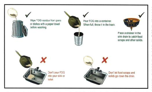
A byproduct of cooking, FOG comes from meat, fats, lard, oil, shortening, butter, margarine, food scraps, sauces, and dairy products. When washed down the drain, FOG sticks to the insides of sewer pipes. Over time, FOG can build-up, block entire pipes, and lead to serious problems. To prevent any undue introduction of FOG into the wastewater collection system, the City of Mebane implements a FOG Policy designed to
