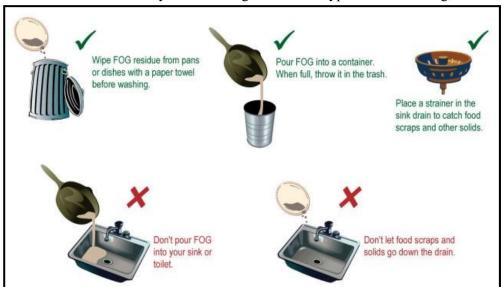
lard, oil, shortening, butter, margarine, food scraps, sauces, and dairy products. When washed down the drain, FOG sticks to the insides of sewer pipes. Over time, FOG can build-up, block entire pipes, and lead to serious problems. To prevent any undue introduction of FOG into the wastewater collection system of the City.
