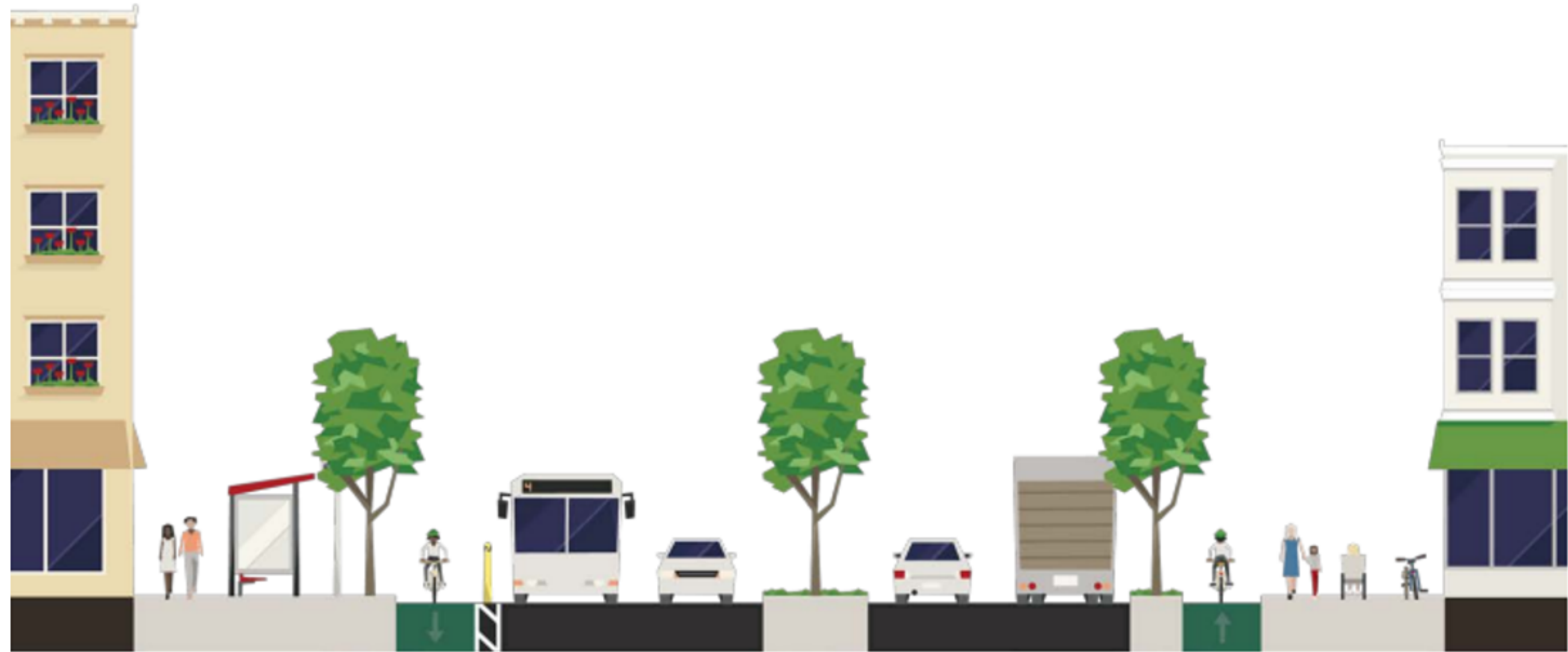
Arterial–Boulevard Typical Section Example 2: Mixed Use Arterial–Boulevard with Median and Protected Bike Lanes
