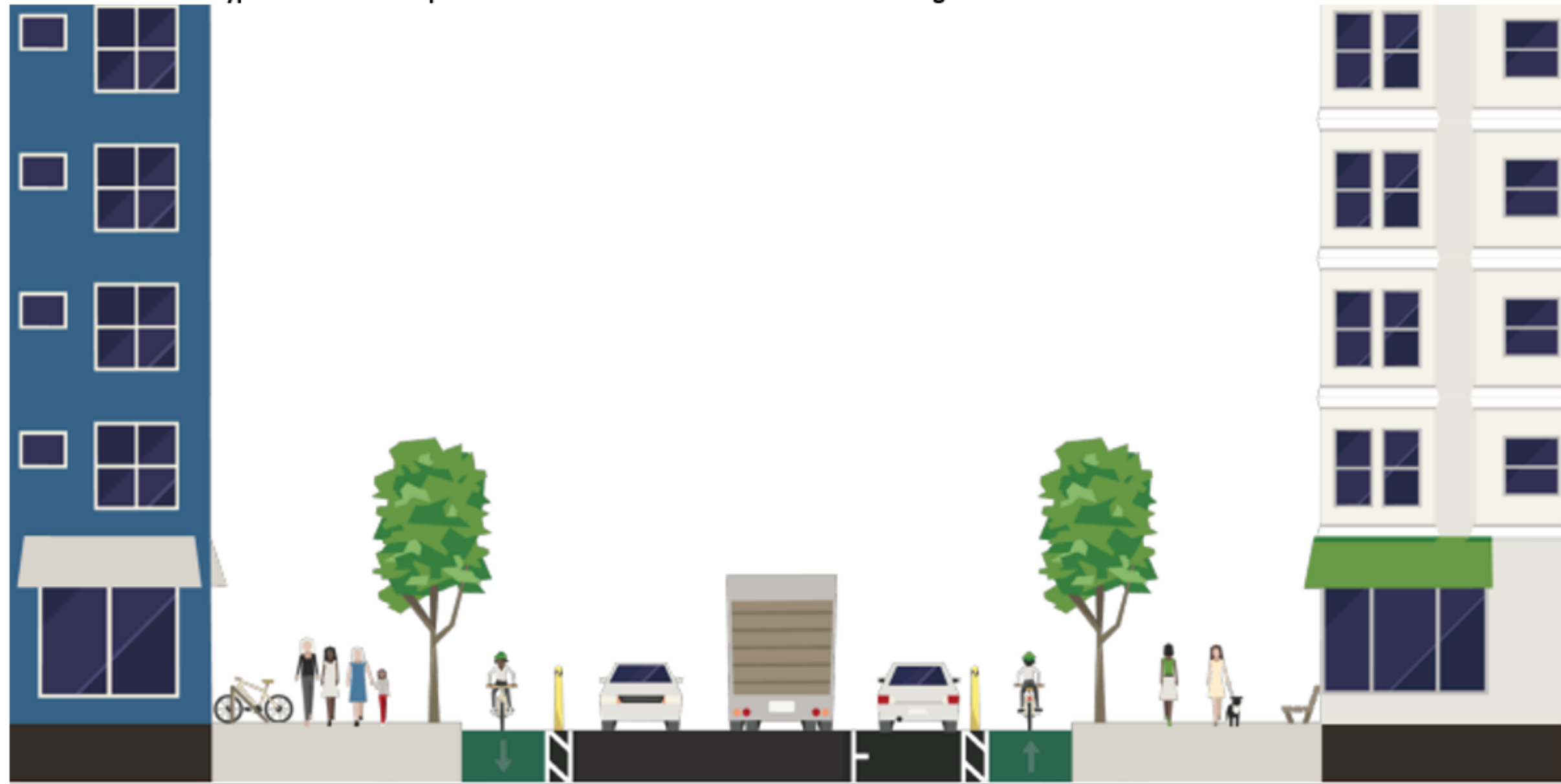
Arterial–Boulevard Typical Section Example 5: Mixed Use Arterial–Boulevard with Parking and Protected Bike Lanes
