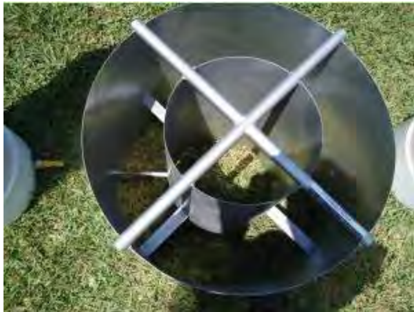
Figure VII.6. Photo of Pre-fabricated Double Ring Infiltrometer
