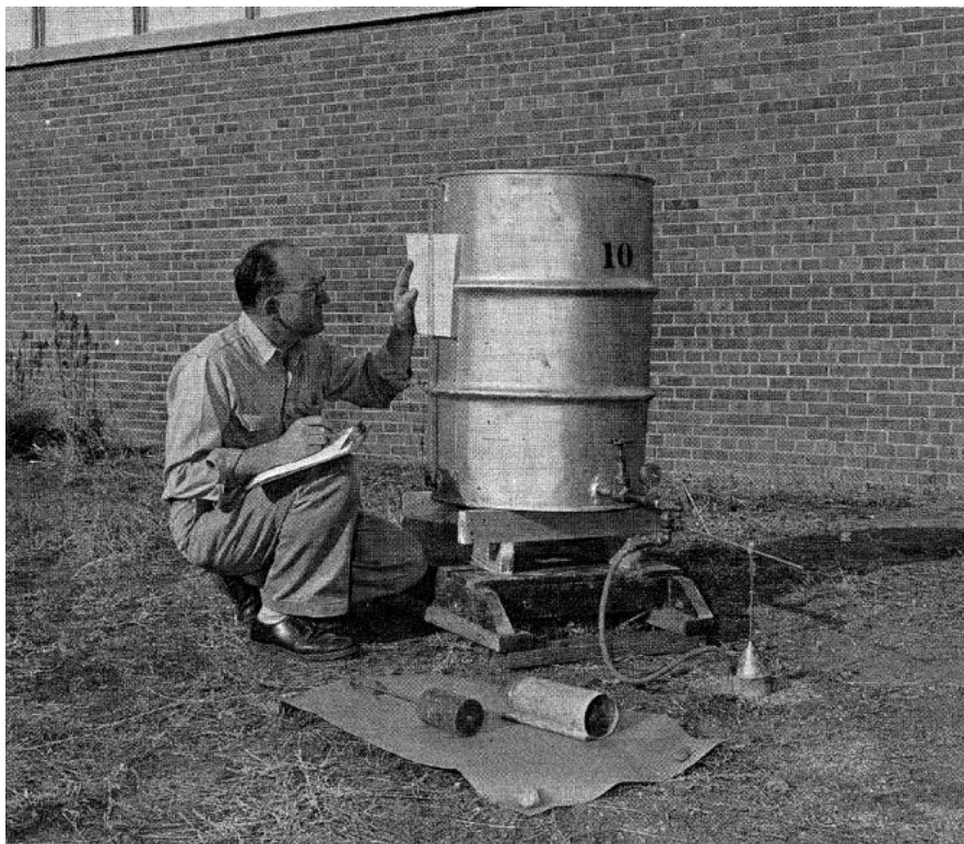
Figure VII.13. Typical Well Permeameter Test Installation
