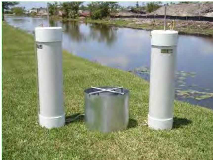
Figure VII.10. Double Ring Infiltrometer Set-up with Mariotte Tubes
