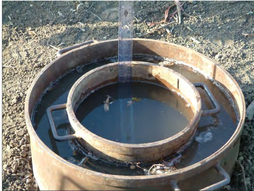
Figure VII.5. Photo of Simple Double Ring Infiltrometer
