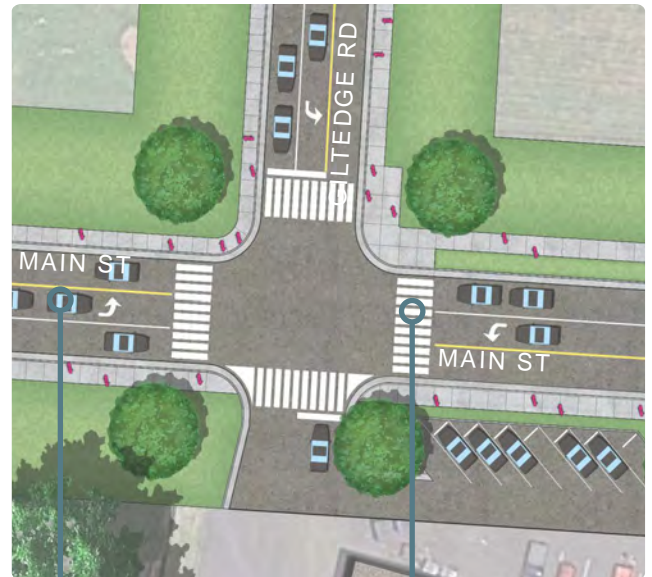
Turn lanes improve intersection functionality and safety
