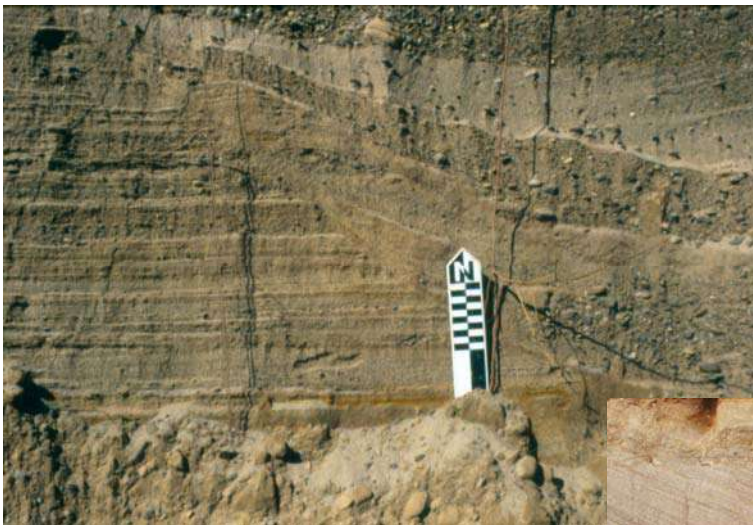
Typical till in northeast Ohio has a high proportion of clay, with silt, gravel, cobbles, and boulders mixed in. Source: J Szabo, University of Akron.
