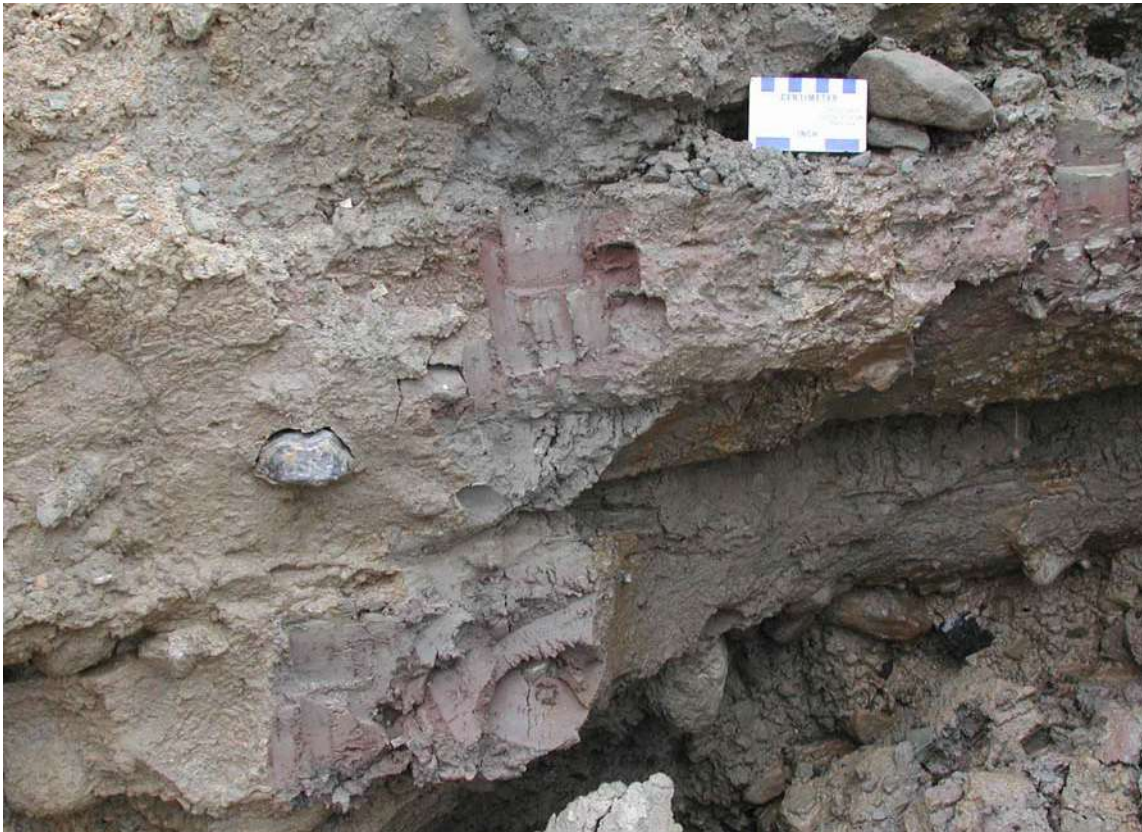
Typical till in northeast Ohio has a high proportion of clay, with silt, gravel, cobbles, and boulders mixed in. Source: J Szabo, University of Akron.
