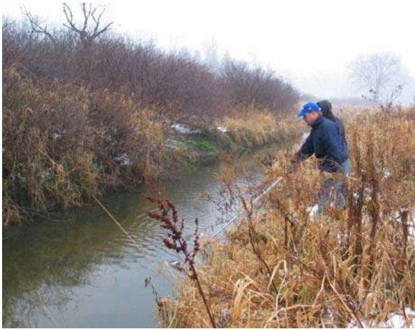
Po-070 Potter Creek, site of potential over-wide ditch design to restore flood storage and a narrower, sinuous channel. Site received low QHEI score due to embeddedness, poor channel form, lack of sinuosity and cover. Dec., Oct., 2007.
