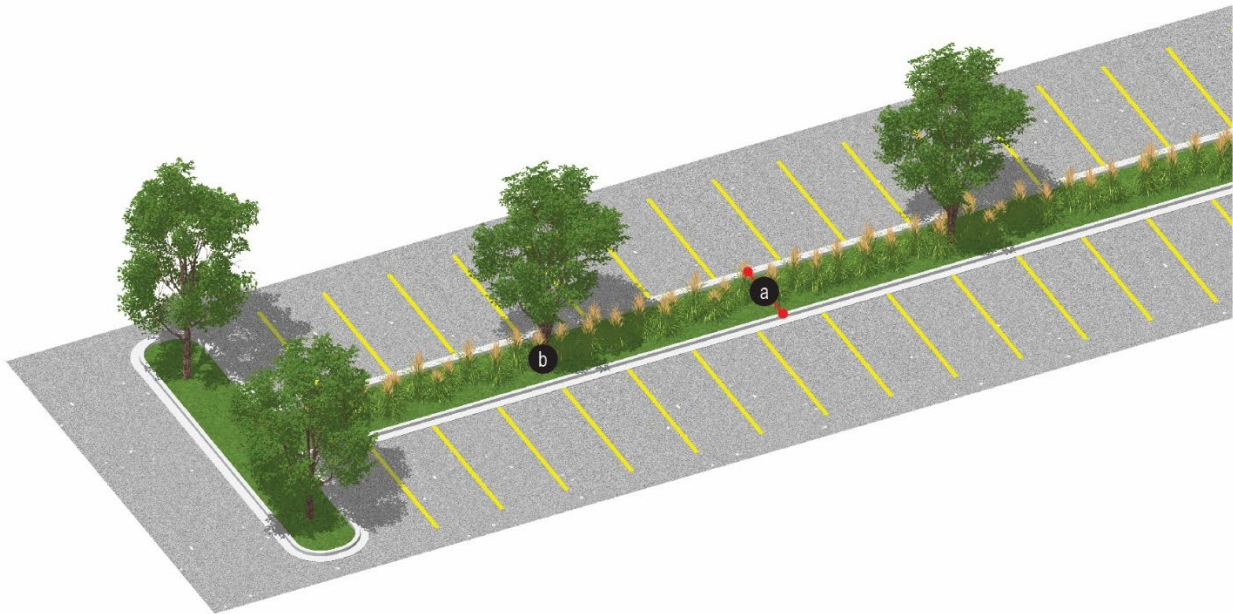
Figure 5.13. Parking Area Median Standards
