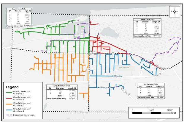
Note: pressurized sewer main is not part of the project scope, it is only listed on the above map for reference purposes.
