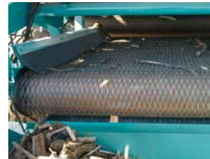
❹ 2-belt screening system The 2-belt screening system guarantees optimum sifting of the sand.
