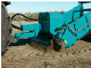
❶ Working width Working width of 1.85 m for coverage of up to 22,000 m 2 /h
