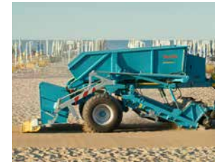
❺ Collecting tank The collecting tank of 0.7 m 3 is emptied into the dumper.
