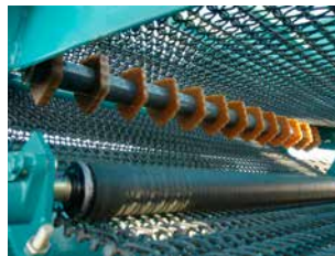
❸ Tension roller Tensioning of the screening belt prevents a loss in performance.
