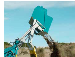
❺ Collecting tank The collecting tank has a loading volume of 1.5 m 3 . Unloading height of 2.60 m (in DIN containers or directly onto a truck).
