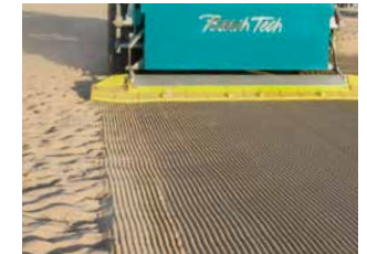
❻ Finisher To structure, aerate and then compress the sand.
