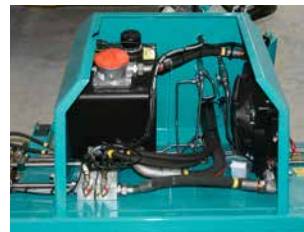
❹ Under the hood Tank, radiator and control block are quick and easy to access for all inspection and service work.
