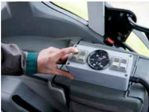
❶ 1-man operation Control of all working processes via remote control in the driver's cab
