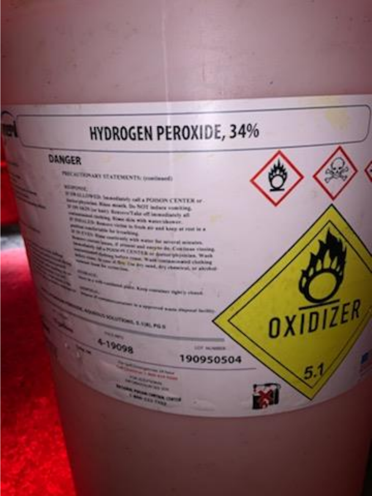
The water system uses hydrogen peroxide as a sanitizer.
