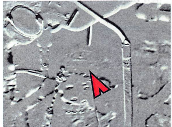
No. 4 Leak observed at a subgrade leak on Well L in High Sensitivity Mode.
