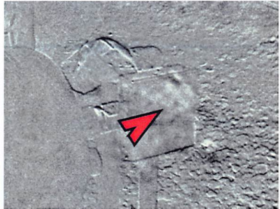
No. 10 Leak observed at an actuator on Separator F in High Sensitivity Mode.
