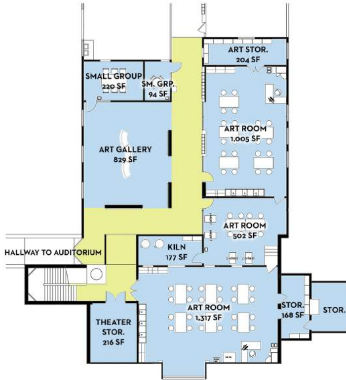
SECOND FLOOR PLAN VISUAL ARTS RENOVATION
