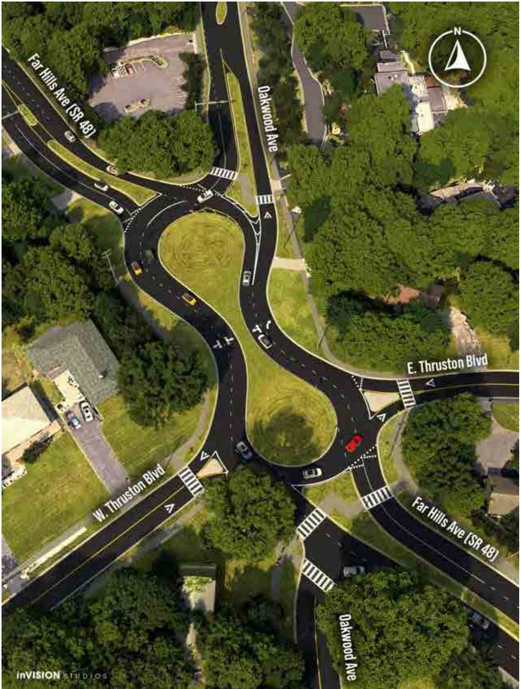
FIGURE 14: ROUNDABOUT CONCEPT PLAN
