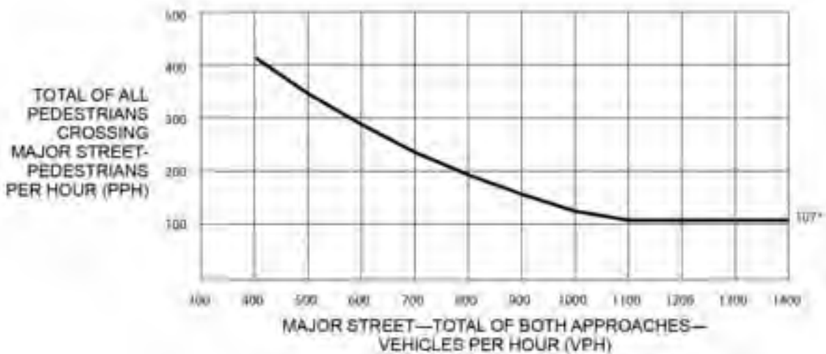
FIGURE 4: OMUTCD FIGURE 4C-5 WARRANT 4, FOUR-HR PEDESTRIAN VOLUME
