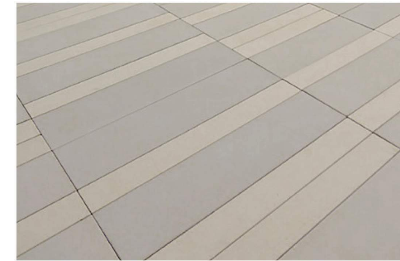
P3 CONCRETE PAVER - TYPE 2 MATERIAL: PRECAST CONCRETE, MORTAR SET SIZE: WIDTHS 6"/12"/24", LENGTHS 48"/60" COLOR/FINISH: LIGHT BUFF/TAN, SANDBLAST
