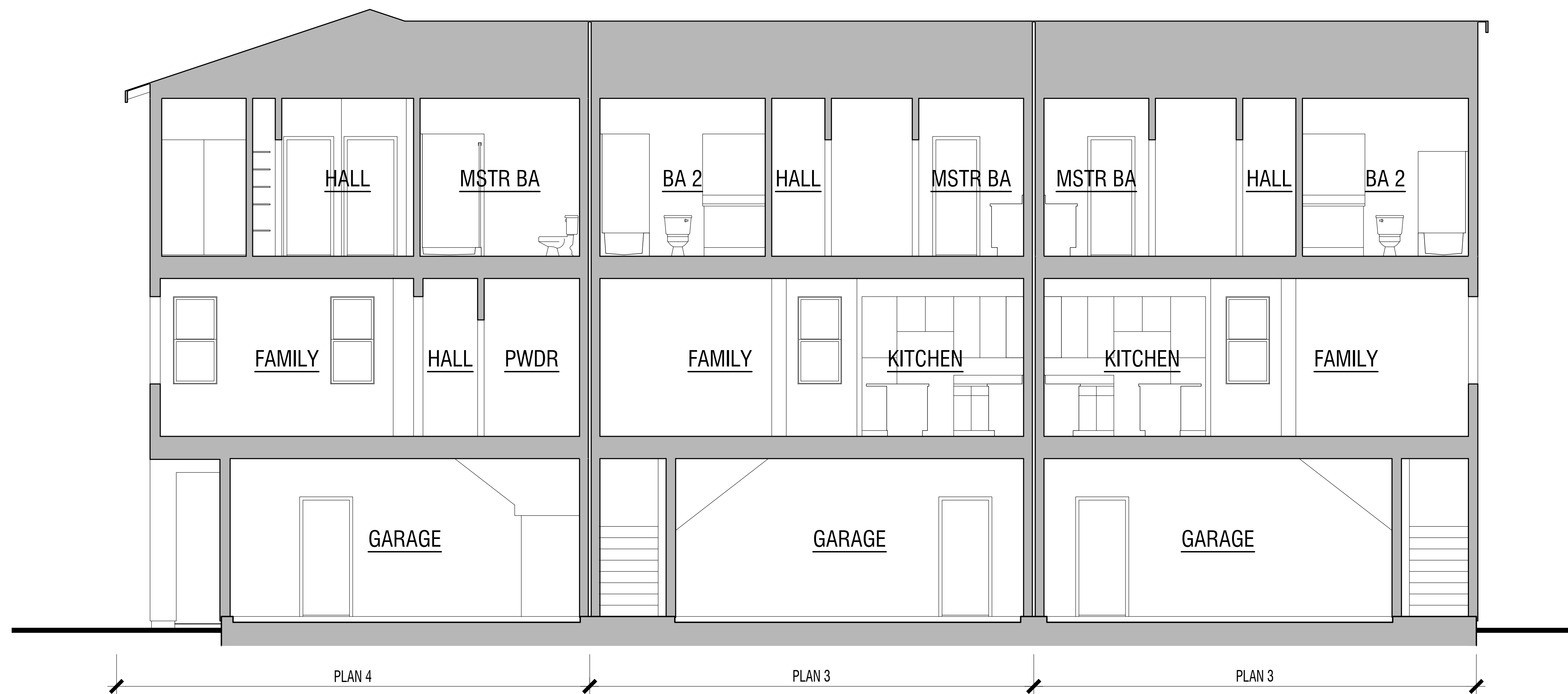
Building Section B-B - Building B
