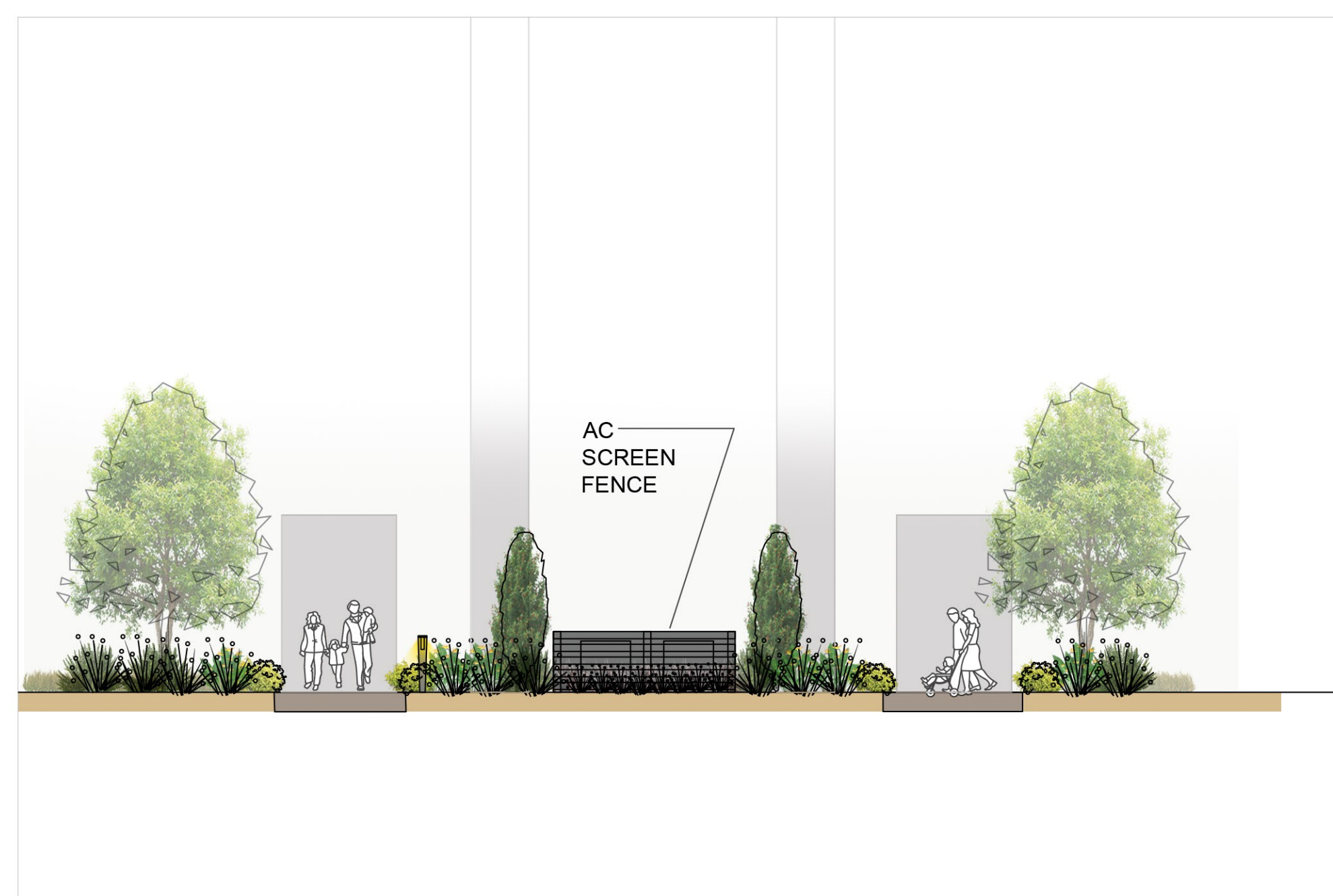
AC UNIT SCREEN FENCE (ELEVATION) SCALE: 1/8" = 1'-0"
