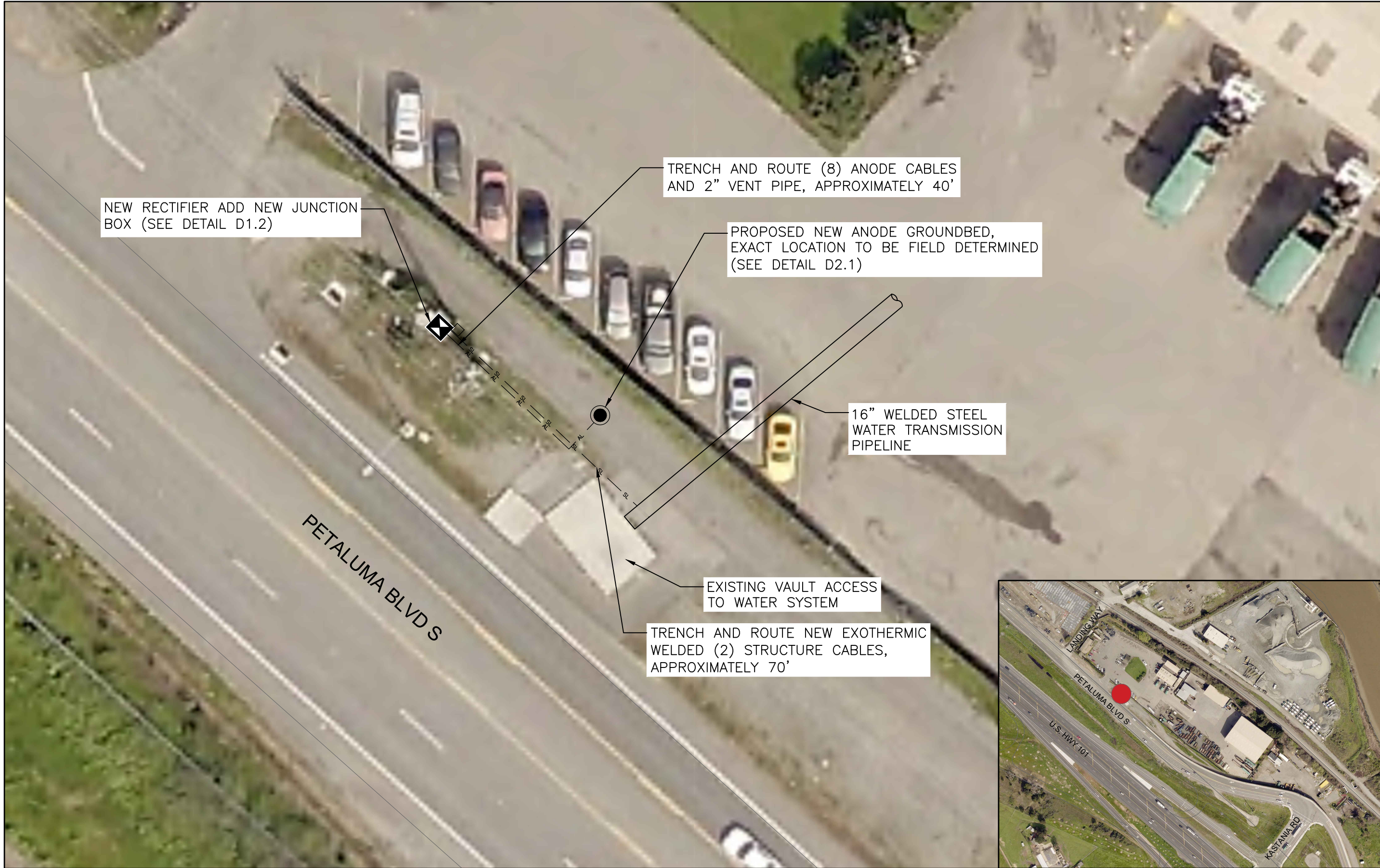
C1.1 RECTIFIER, JUNCTION BOX AND DEEP ANODE GROUND BED GPS: 38.223031, -122.609298
