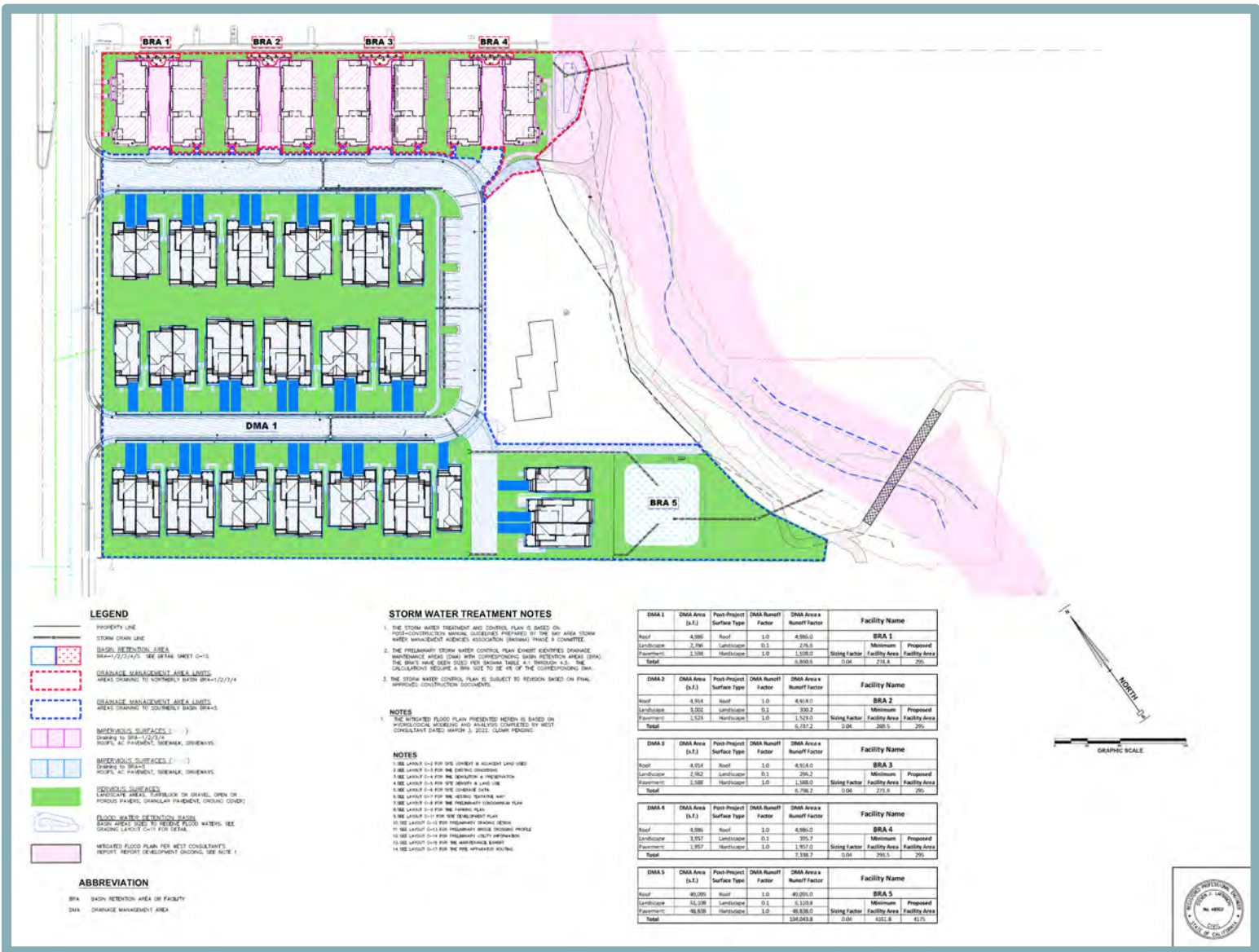
Figure 8 Post-Construction Stormwater Control and Treatment Plan
