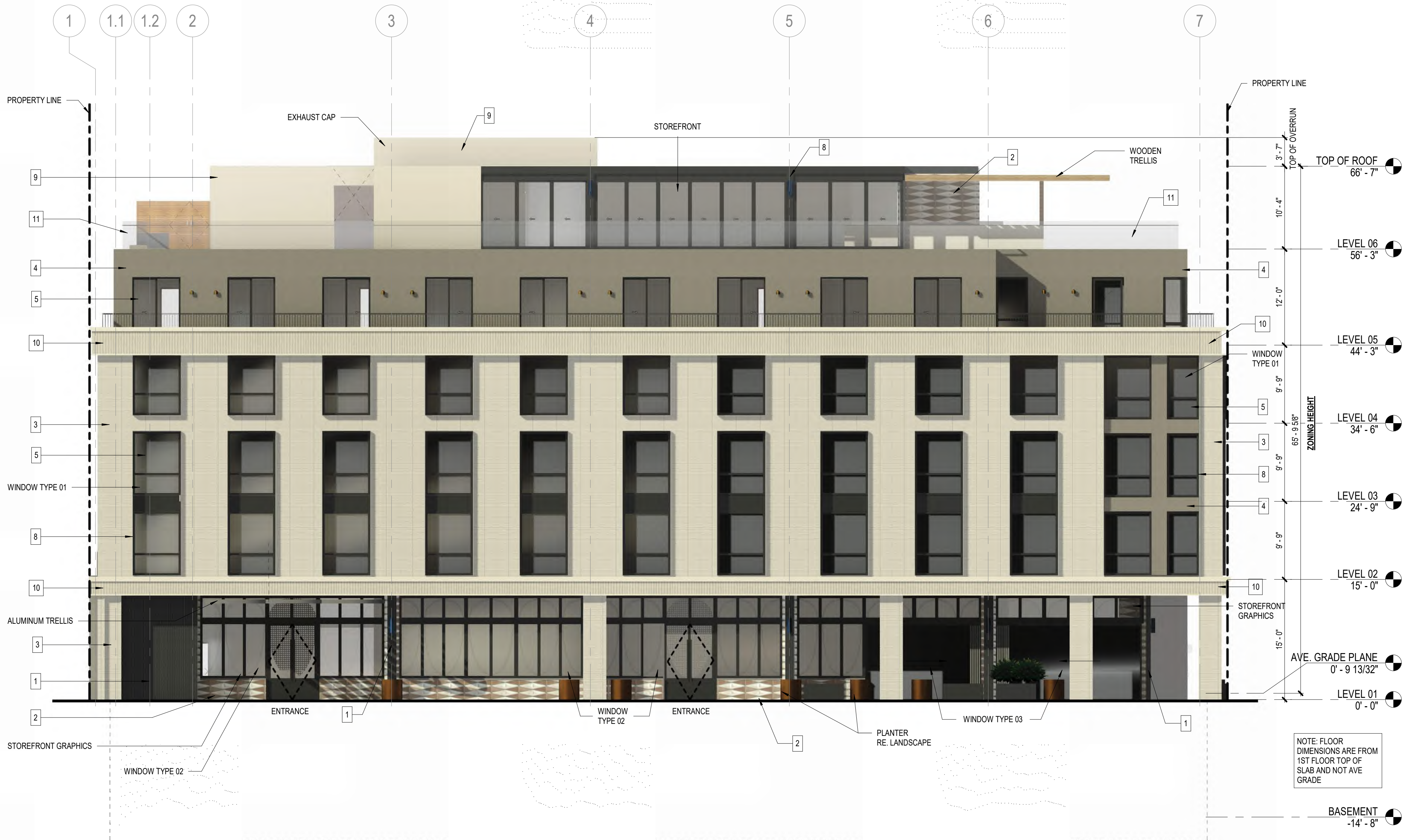
1 ELEVATION - MAIN ENTRY - NORTH SCALE: 1/8" = 1'-0"
