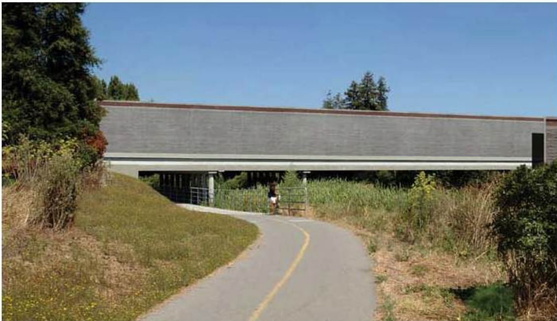
Figure 3.1-53 Proposed Lynch Creek Bridge with Soundwall
