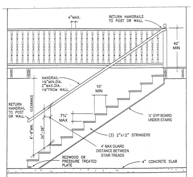
All stairs having four or more risers are required to have handrails and guardrails that comply with the current code. See the 2013 California Residential Code Sections R311.7.8 and R312.
