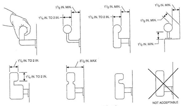
NOTE: Other shapes may be acceptable if they provide an equivalent gripping surface. See third paragraph of Section 1003.3.3.6.
