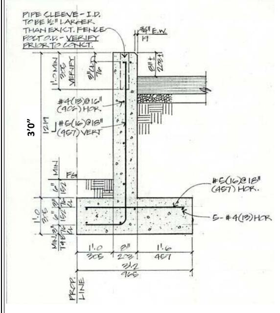
S:\BUILDING\Forms\2013 Building Handouts\Retaining Wall Detail.doc
