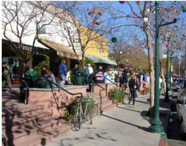
A raised Dooryard along a series of commercial spaces provides seating areas outside of the public path of travel
