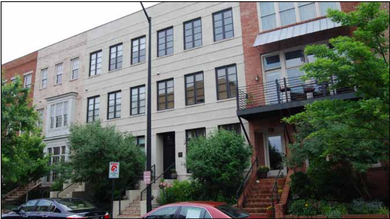
Different materials window treatments applied to a simple facade plan articulate the individual townhouse units.
