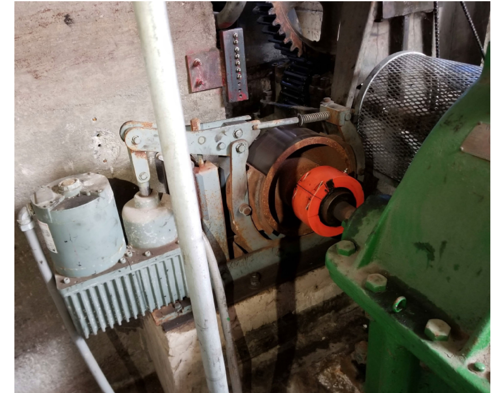
MAIN MOTOR BRAKE THRUSTER ASSEMBLY
