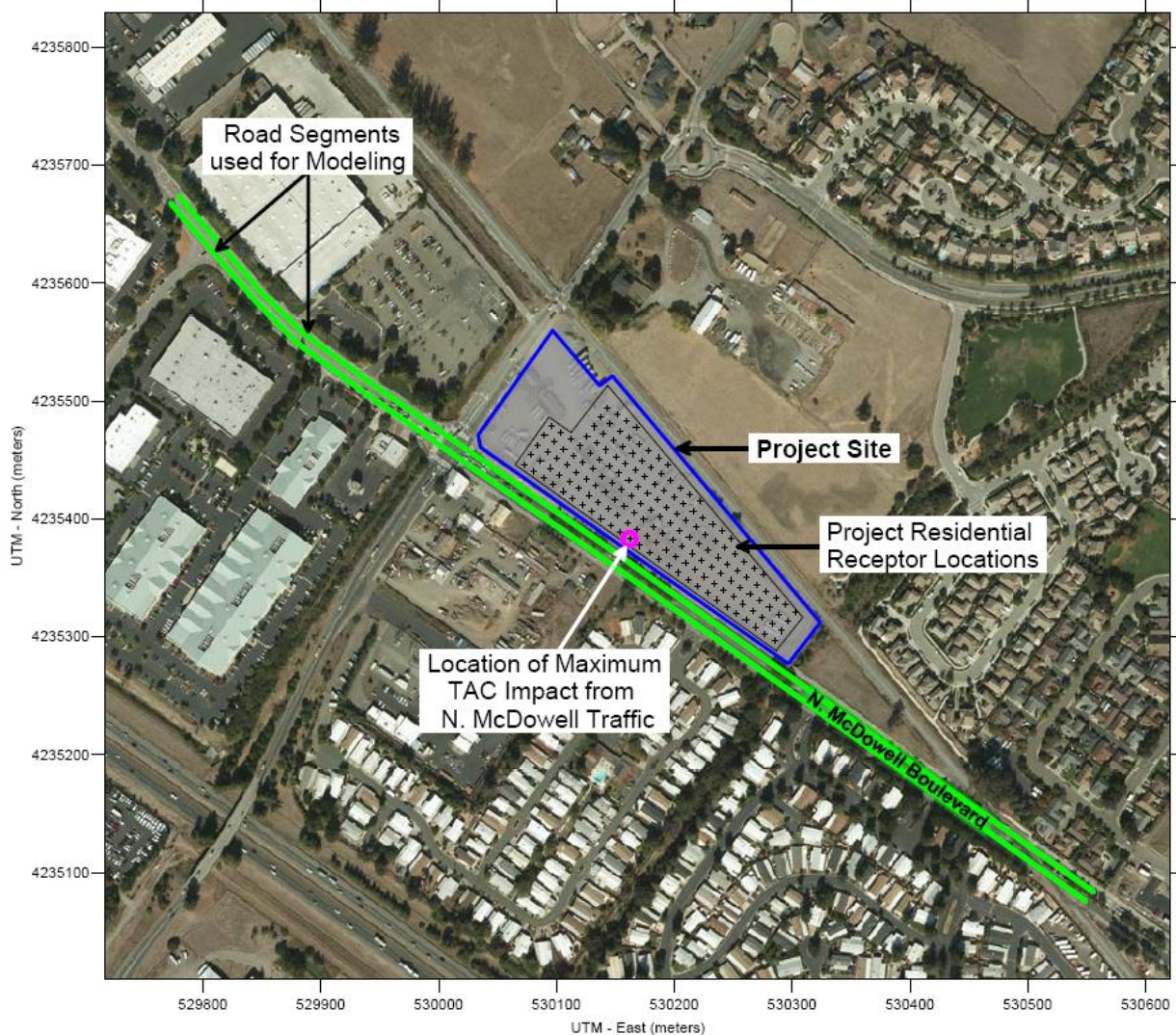
Figure 1. Project Site, On-Site Sensitive Receptors, Roadway Segments Modeled and On-Site Receptor with Maximum TAC Impacts
