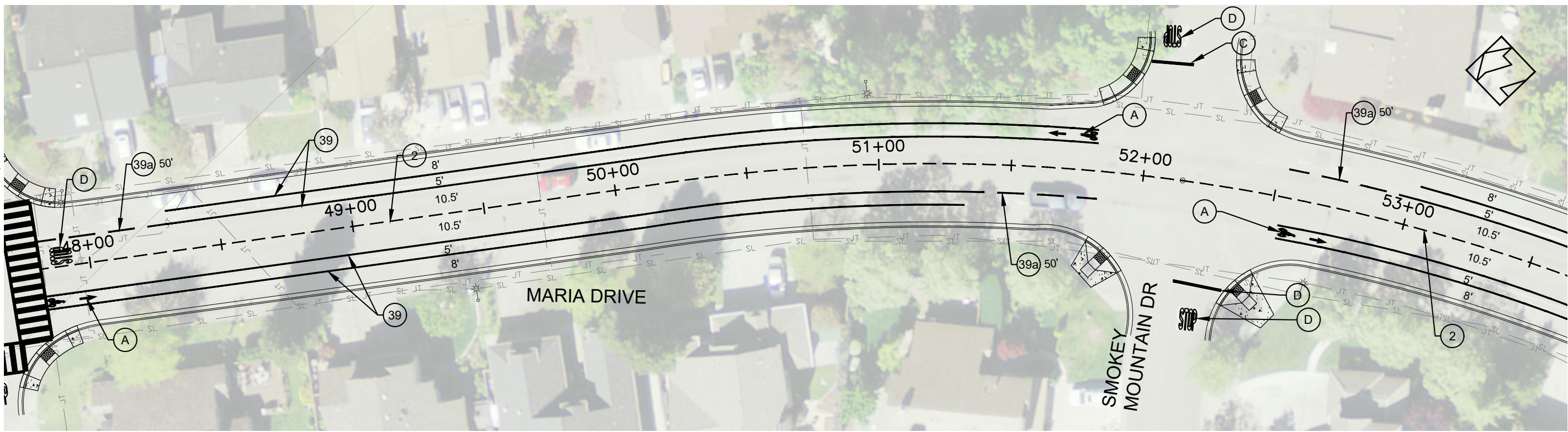
STRIPING - MARIA DRIVE STA 48+00 TO STA54+00
