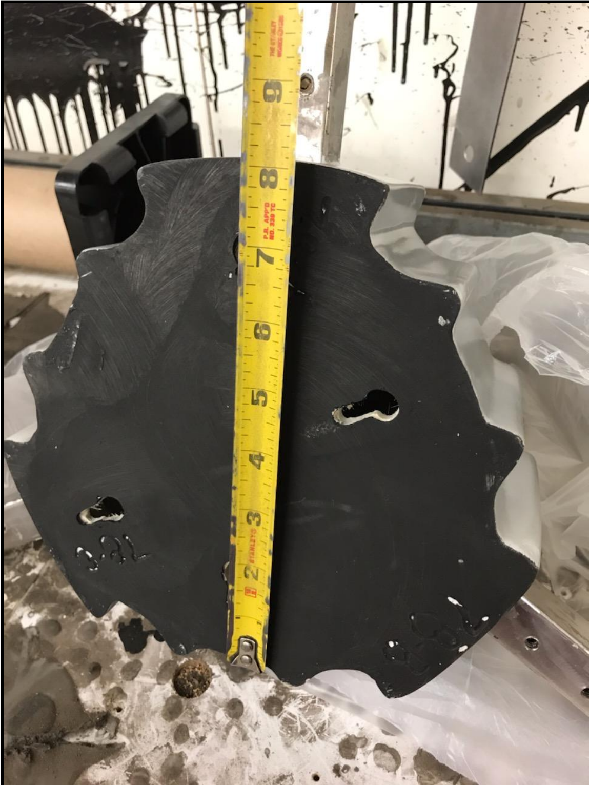
Figure 3: Image of propeller hub backside, vertical dimensions.
