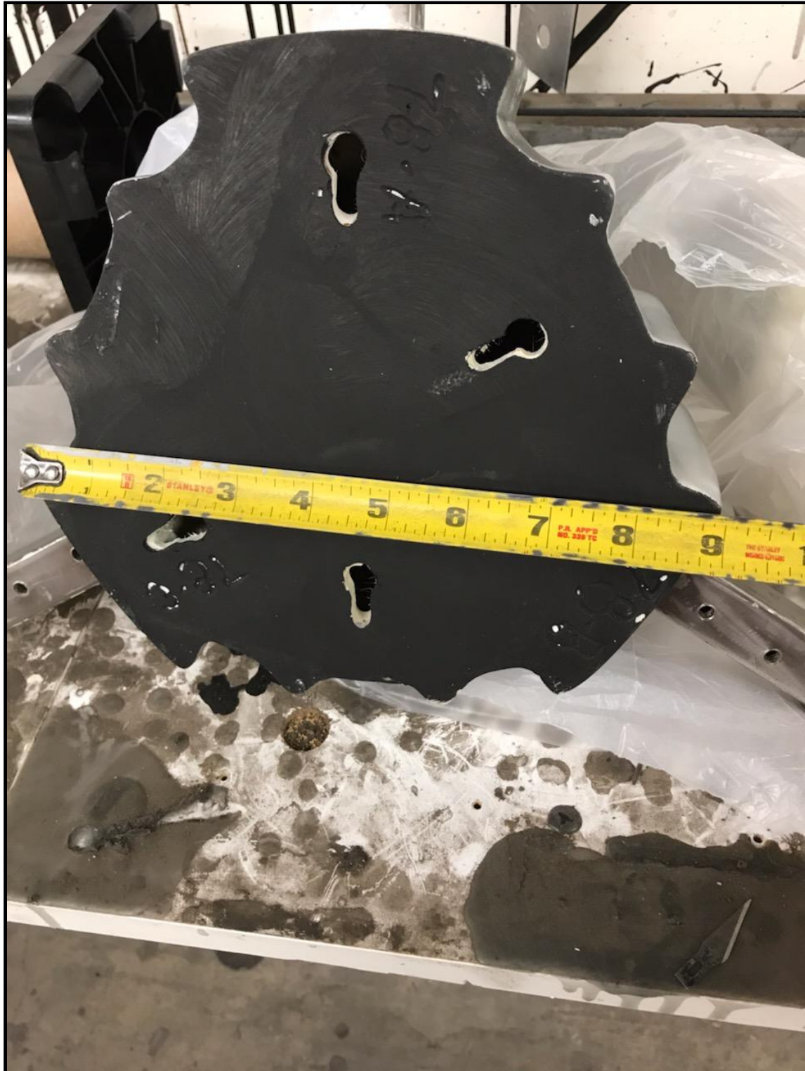
Figure 2: Image of propeller hub backside, horizontal dimensions.
