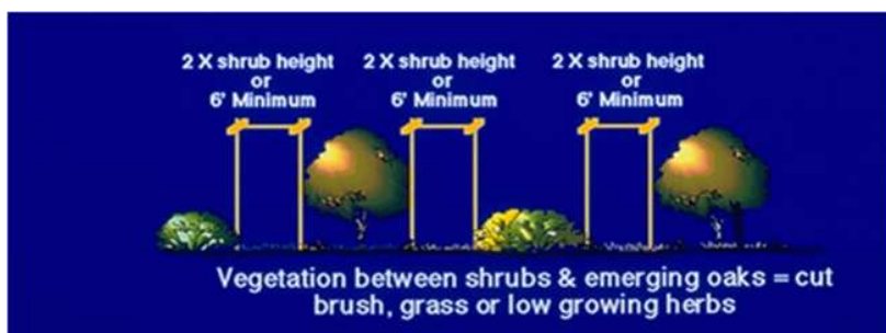
Figure 10. Shrub island spacing. Design groups of plants small enough to provide horizontal separation between groups. This allows proper maintenance and helps slow the spread of fire. Each shrub or group of plants should measure no wider than two times its height, or less than 120 sq. ft. (or 6 ft x 20 ft). The space between groups should be greater than three times the height of the shrubs, or at least a 12 ft. distance
