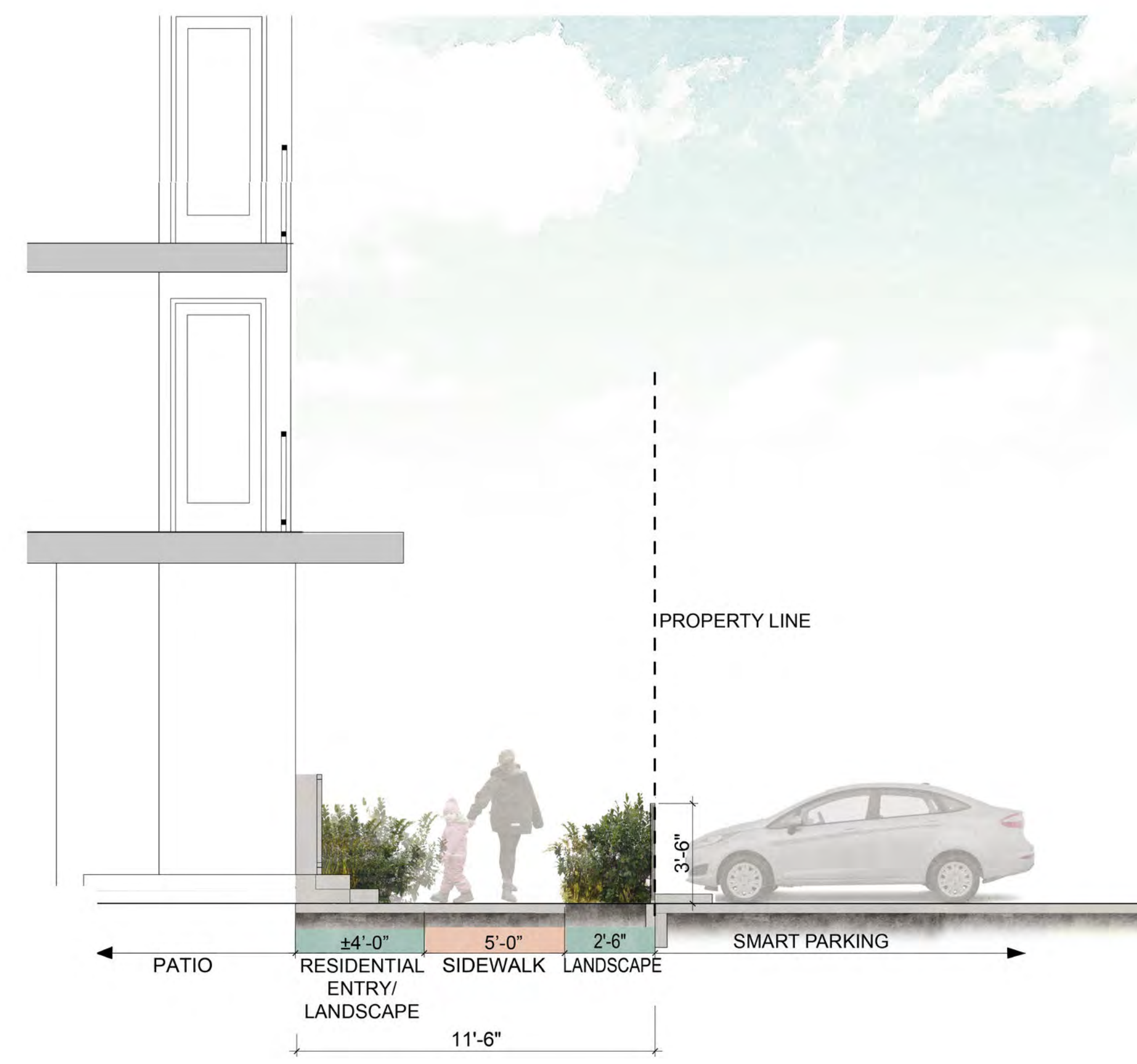
Section G-G' SMART STATION
