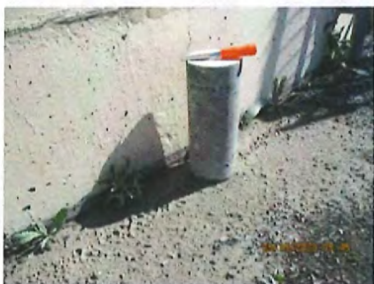
6" concrete core sample for checking interior liner.
