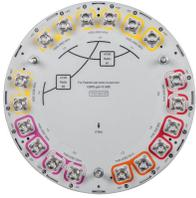
18-port small cell antenna, 4x 698-896, 8x 1695-2690, 4x 3400-3800 and 2x 5150-5925 MHz, 360° Horizontal Beamwidth, fixed tilt.
