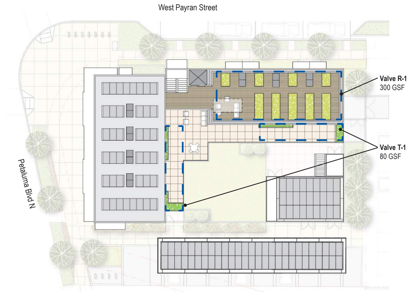
Roof and Second Level - Hydrozone Diagram
