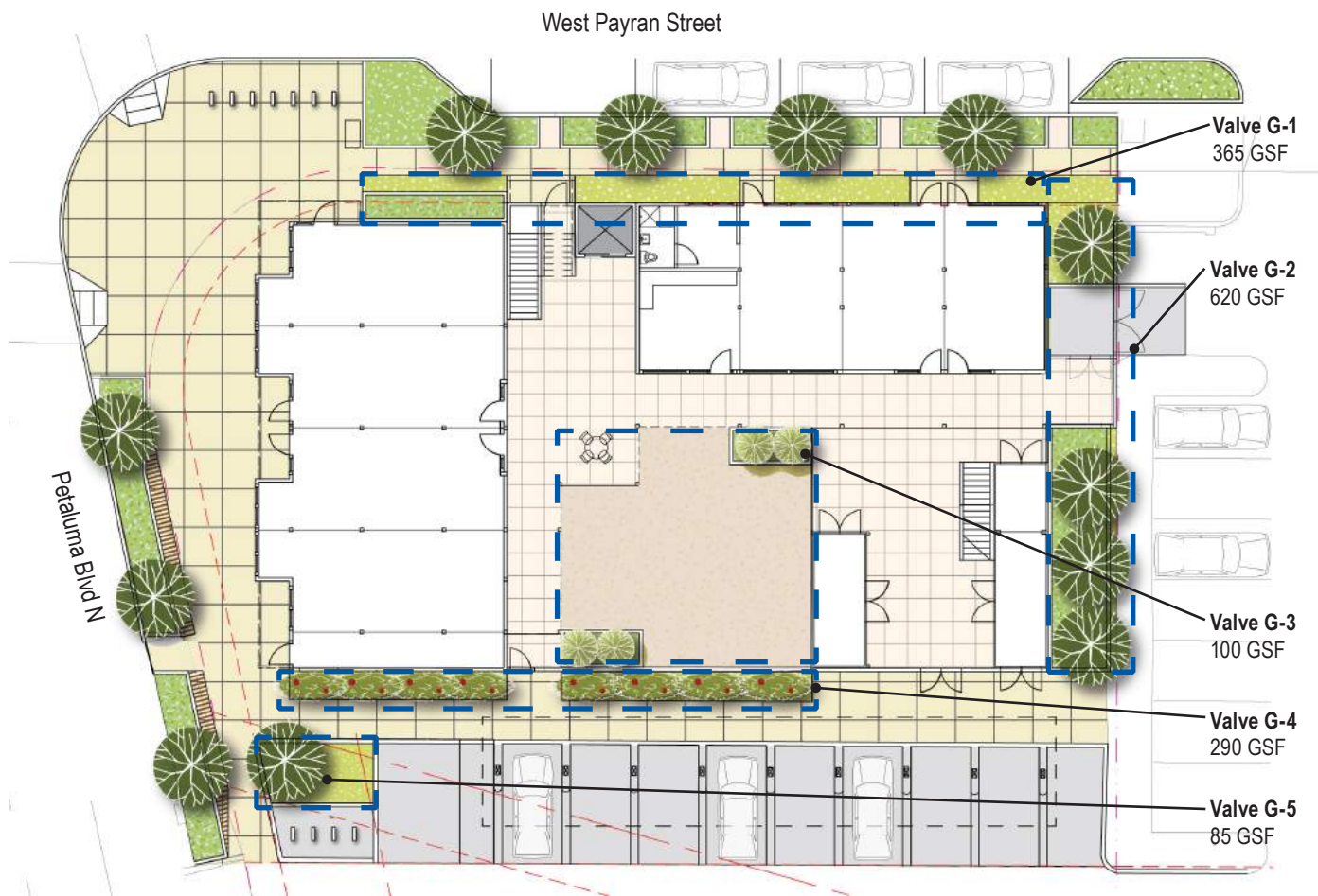
Ground Level - Hydrozone Diagram
