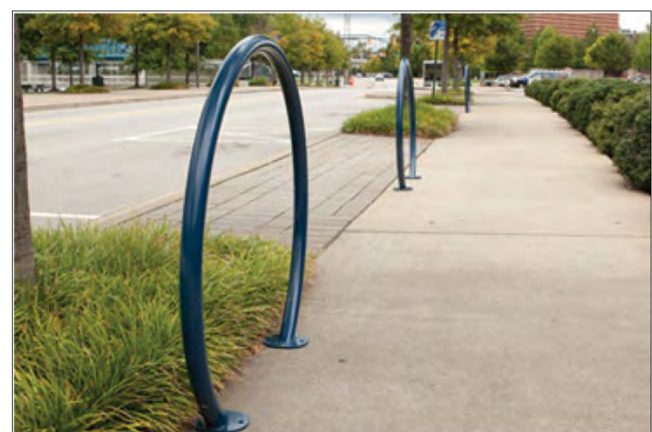
SOLSTIC BIKE RACK (BY MRC RECREATION) CAPACITY: UP TO 2 BIKES OVERALL DIMENSIONS: 37" HIGH X 42" WIDE FRAMEWORK: 1.9" OD X 11 GAUGE PRE-GALVANIZED TUBING MOUNTING OPTIONS: SURFACE MOUNT AND IN-GROUND MOUNT OPTIONS
