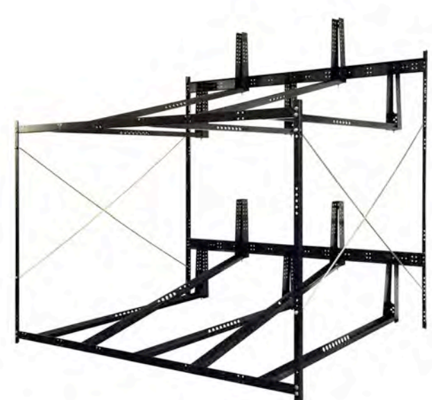
B. STRETCH RACK 8110 (BY SARIS PARKING) CAPACITY: UP TO 10 BIKES OVERALL DIMENSIONS: 72" X 63" X 86" HIGH (WITH BIKES IN) FINISH: POWDER COAT FINISH BLACK MOUNTING OPTIONS: FREE STANDING OR MOUNTED IN WALL OPTIONS
