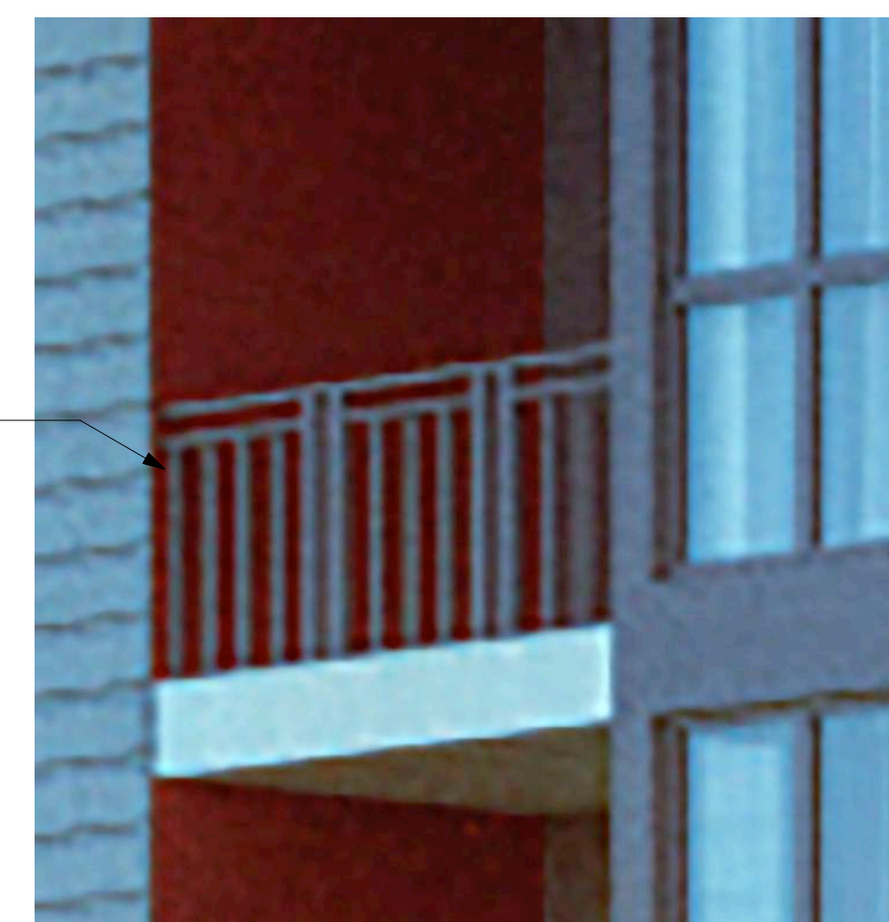
STEEL TUBE RAILING, PAINTED 3 NTS
