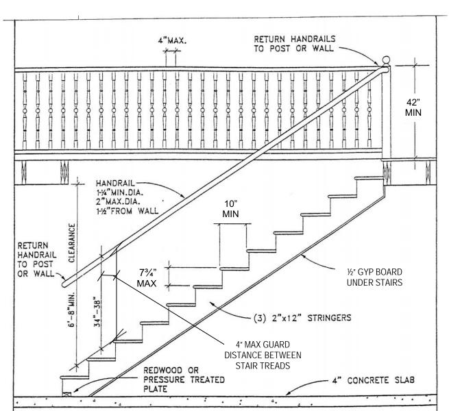
All stairs having four or more risers are required to have handrails and guardrails that comply with the current code. See the 2019 California Residential Code Sections R311.7.8 and R312.
