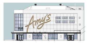
seismic retrofit, adaptive reuse of existing retail space, replacement of three windows, and three new windows below the original windows, a new double-door and infill wall for a side entrance, windows and a door on the West façade, and new signage, as well as various alterations that are proposed for the interior of the building. Building square footage would be expanded to approximately 20,000 SF through the addition of a mezzanine space.
