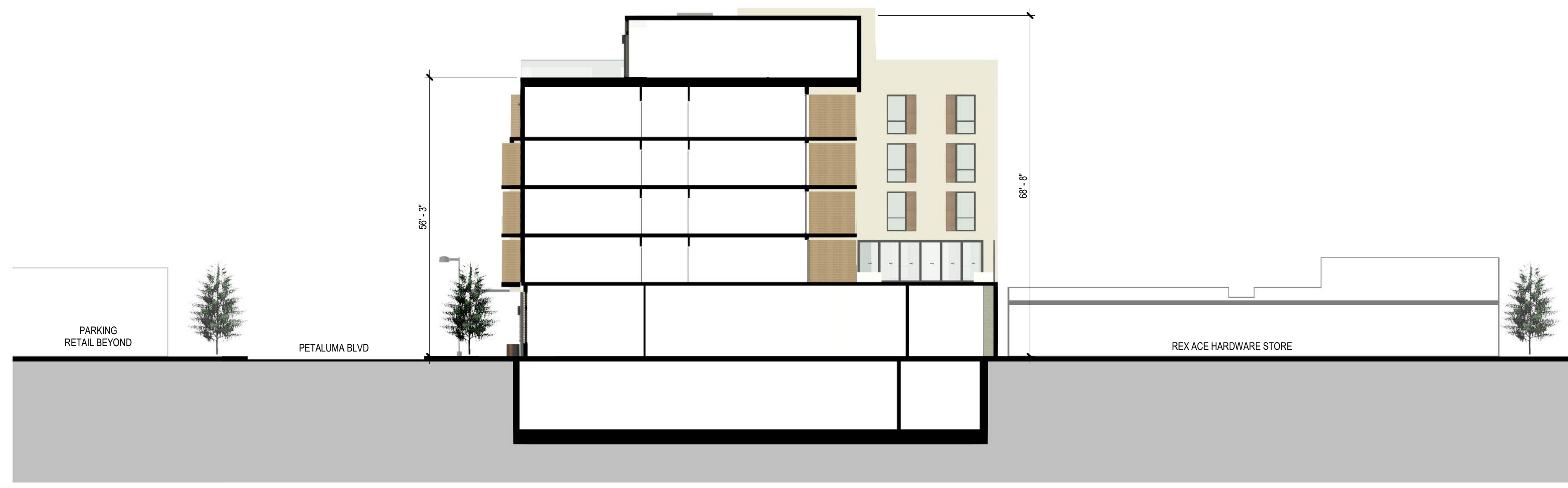
4 SECTION - PETALUMA BLVD SCALE: 1/16" = 1'-0"
