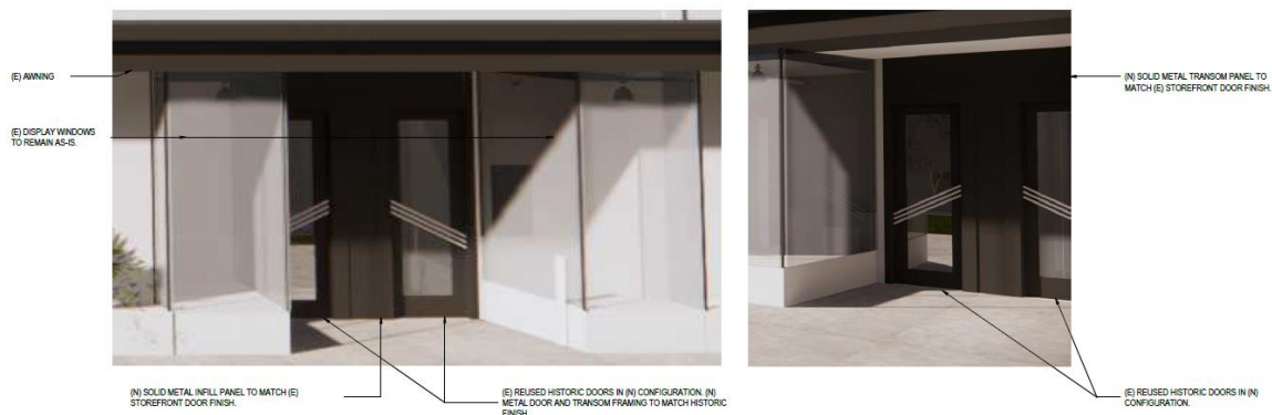
Figure 22. Proposed fire exit door at existing entrance on Kentucky Street. Quezada Architects, “Amy’s Kitchen: Site Plan & Architectural Review” (May 6, 2022), SPAR-203.
