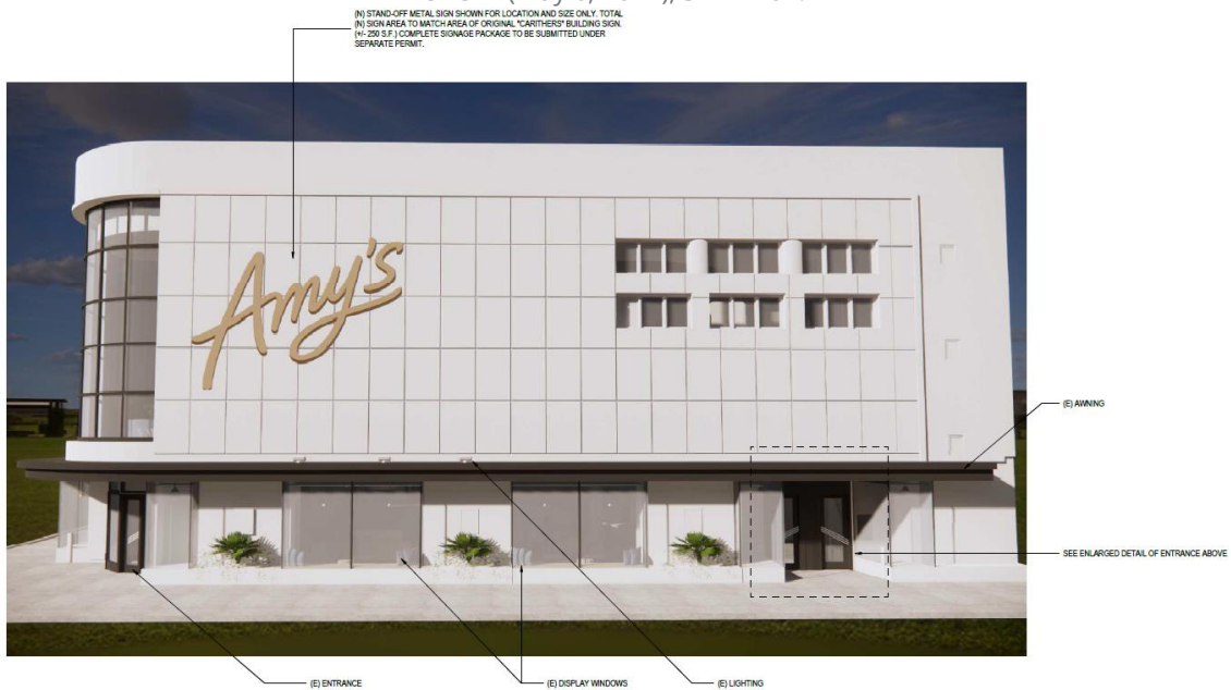
Figure 20. Proposed new windows and metal signage at the east façade. Matching windows will be at the south façade, but the signage will only be located at the east façade. Source: Quezada Architects, "Amy's Kitchen – Site Plan & Architectural Review" (May 6, 2022), SPAR-203.
