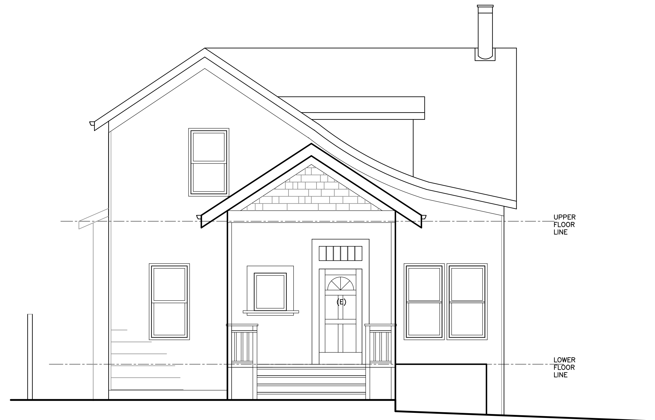
EXISTING WEST ELEVATION
